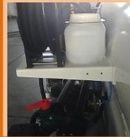
Sanitary concentrate tank capacity 5 l
