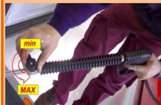
Double barrel spraygun allows the regulation of the washing pressure
